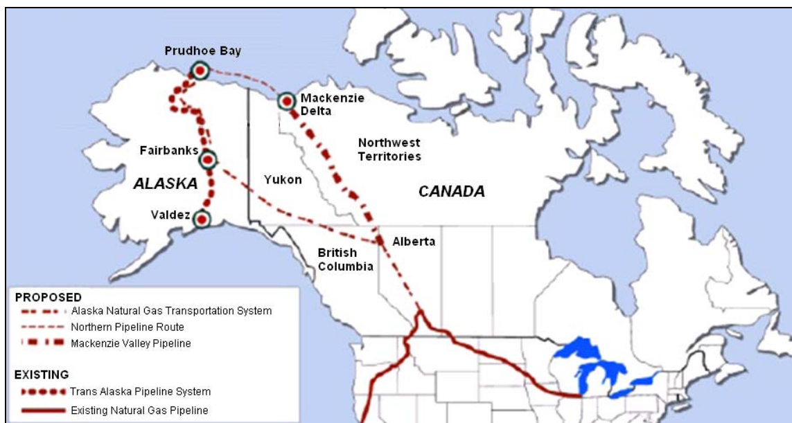
Figure 5. Arctic Natural Gas Pipelines Proposals
