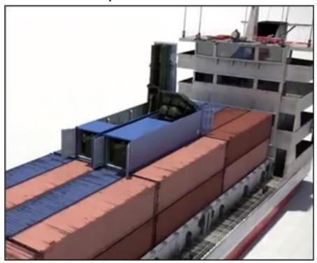
Figure 12. Illustration of Reported Potential Containerized ASCM Launcher
