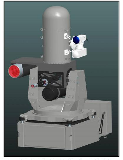
Figure C-2. Rendering of LaWS Integrated on CIWS Mount
