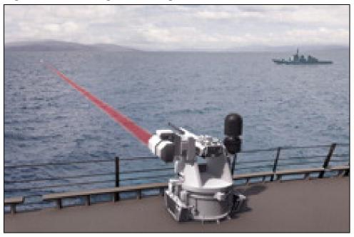
Figure D-I. Rendering of TLS Integrated on Mk 38 Machine Gun Mount
