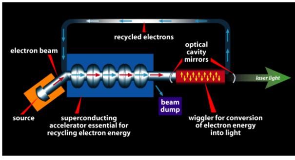
Figure F-2. Simplified Diagram of How an FEL Works
