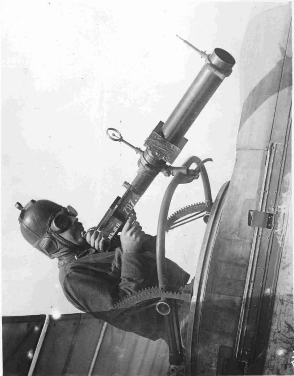
11497 - Apparatus with which experimental or training work was conducted came under the ban. This picture shows <sup>the</sup> Scharf mounted visible gun camera, similar to the Lewis gun, used by the Air service for training flyers in aerial gunnery at Ellington Field, Houston, Texas. May 1918.
