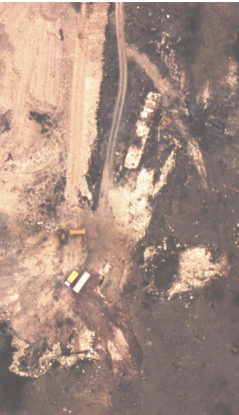
▲ Degelen Mountain: high-resolution aerial photograph of the tunnel 22 site. Note the roads, spoils (or excavation materials from the tunnel), tanks, trucks, equipment sheds—all of which are subtle indicators of the existence of a tunnel.
