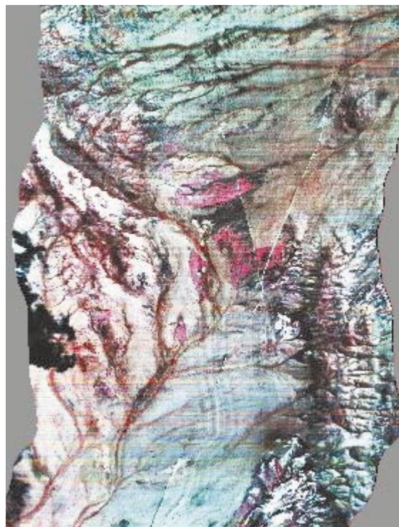
▲ Semipalatinsk Test Site: (top) multispectral image from the Daedalus sensor shows the same area as the photo to the left. (bottom): also the same area, this hyperspectral image is from the CASI. The apparent size reflect the different aspect ratios of the pixels collected by each sensor.
