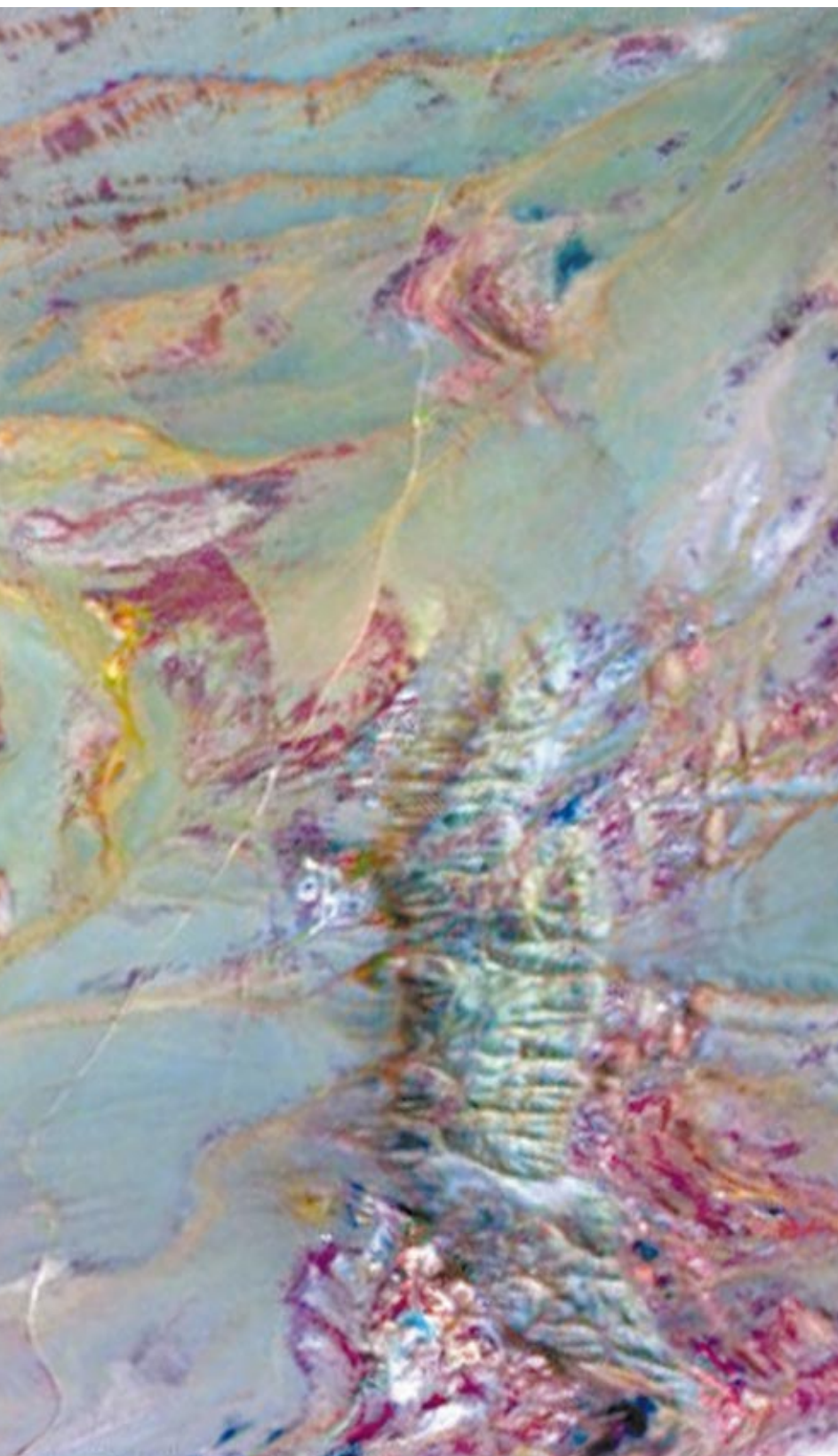
▲ Semipalatinsk Test Site: the Probe 1 hyperspectral image shows high variability in geology and vegetation. Scientists can use this variability to map geologic features and differentiate between mineral types.
