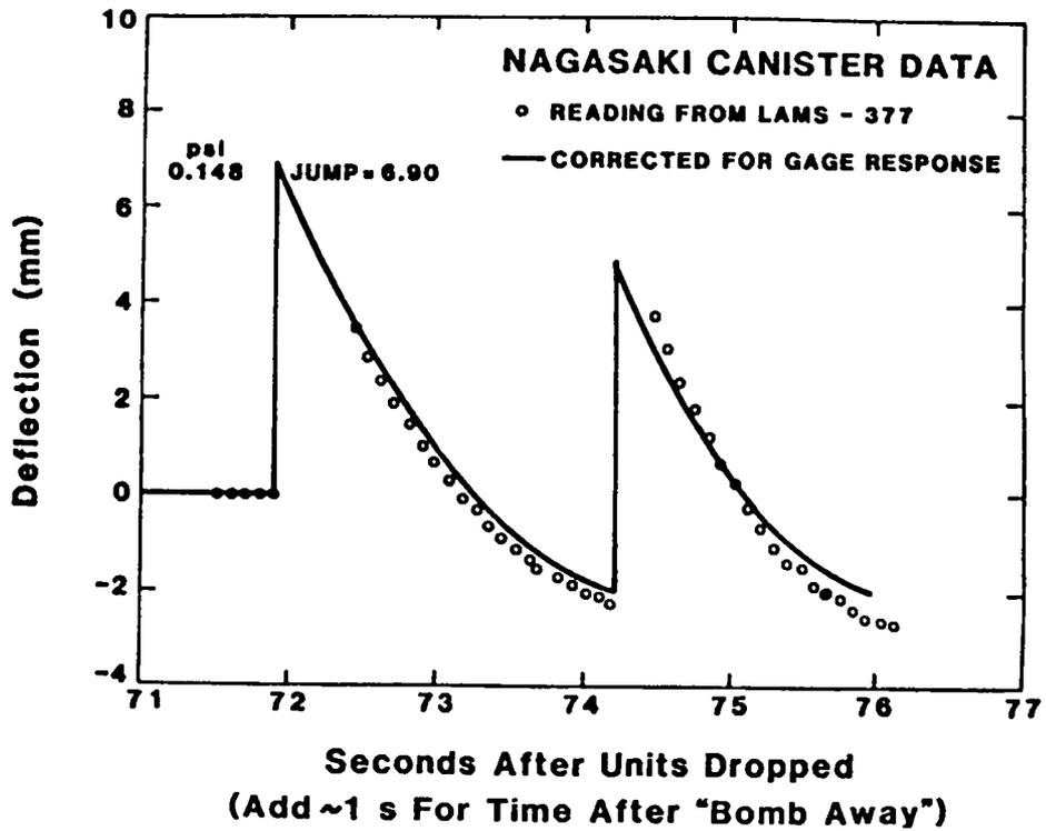
Fig. 2. Nagasaki canister pressure data.
