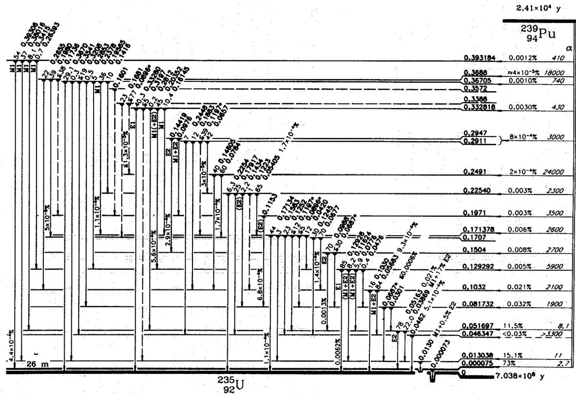
Fig. 1.2 Diagram of some of the nuclear energy levels of <sup>235</sup>U. These levels are populated during the decay of <sup>239</sup>Pu and give rise to the characteristic gamma-ray spectrum of <sup>239</sup>Pu. Figure adapted from Ref. 1.
