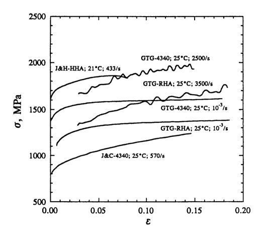
Figure 35. Plot of four different steels on the same axis for comparison. Note that the curve fitting matches only the low strain rate, room temperature data reasonably well.
