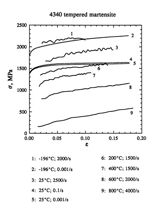
Figure A-1. Raw data for Los Alamos 4340 tempered martensite.
