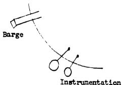
For the lagoon measurements, they would participate in the shot recommended by L\SL as a good one, using a series of stations (probably three, possibly four) which would contain probably six to eight pressuresensing elements per station, and in addition employing ball crusher gauges for peak pressure.
