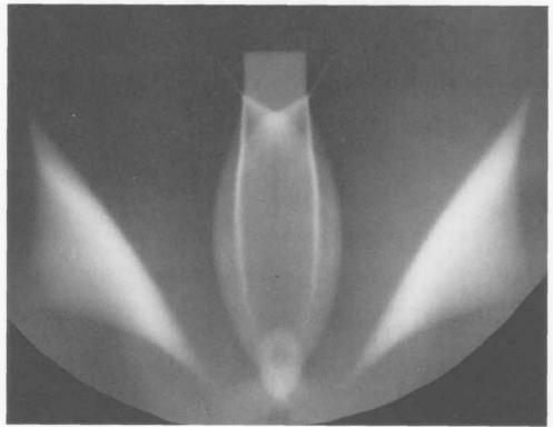
SHOT 1019: Colliding PBX-9404 Cylindrical Detonation Waves
