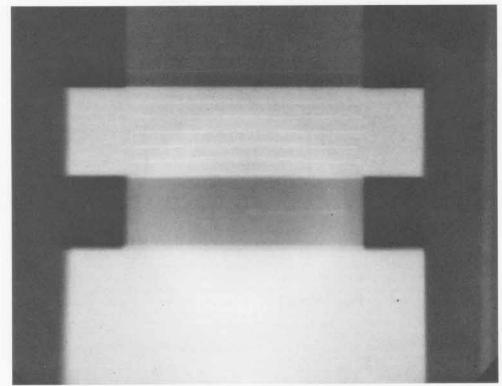
SHOT 1034: Spherically Diverging PBX-9404 Detonation
