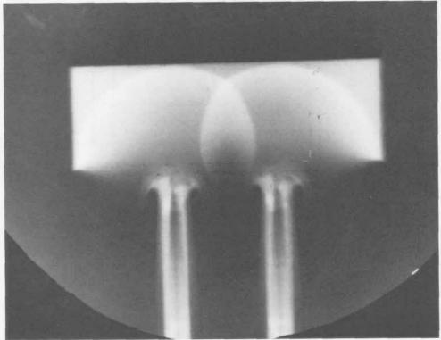
SHOT 1020: Spherically Diverging PBX-9404 Detonation
