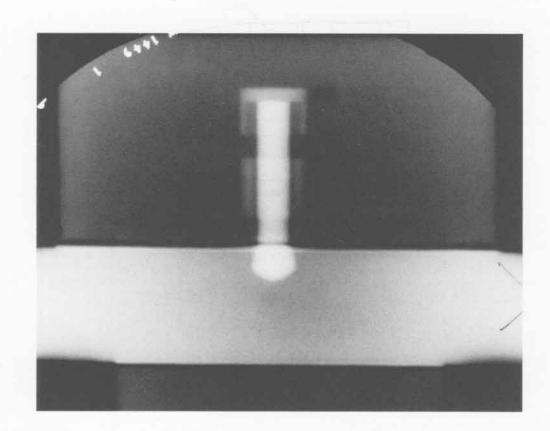
SHOT 1450: Projectile Penetration of a Steel Plate
