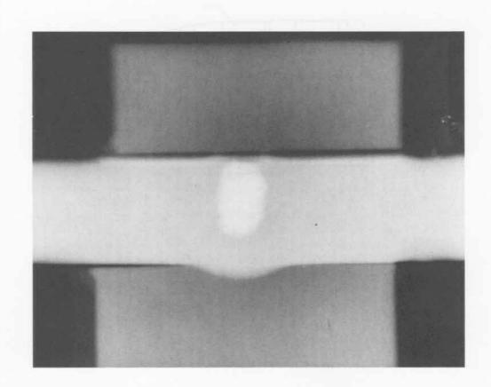
SHOT 1449: Projectile Penetration of a Steel Plate
