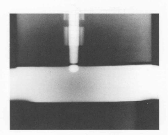
SHOT 1446: Projectile Penetration of a Steel Plate
