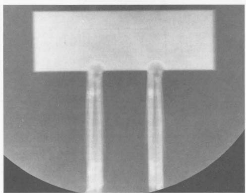
SHOT 1143: Colliding PBX-9404 Cylindrical Detonation Waves
