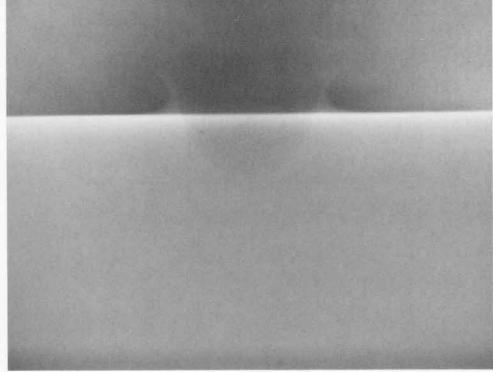
SHOT 1352: Water Splash Wave Formed by a PBX-9404 Sphere
