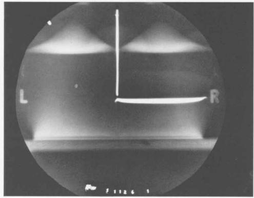
SHOT 1130: Colliding PBX-9404 Cylindrical Detonation Waves
