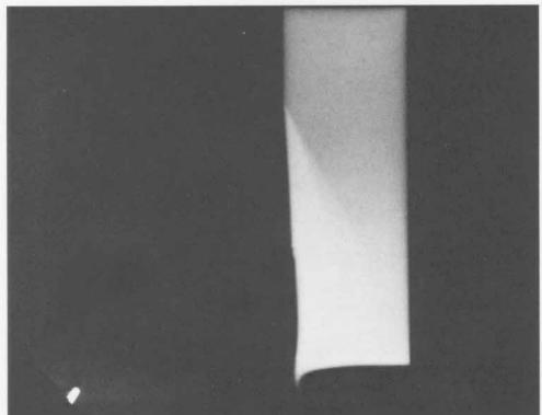
SHOT 988: Spherically Diverging PBX-9404 Detonation
