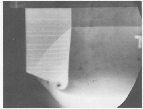
SHOT 1240: Lateral Propagation of PBX-9404 Detonation
