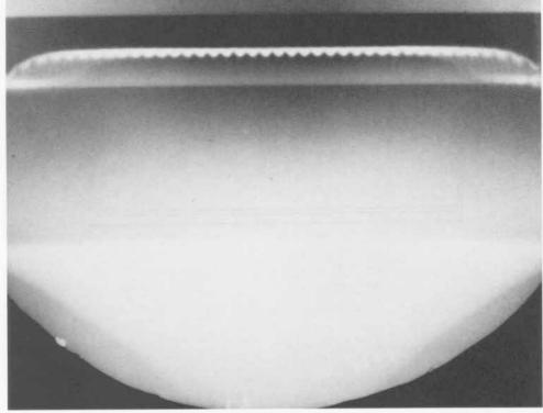
SHOT 1350: Water Splash Wave Formed by a PBX-9404 Sphere
