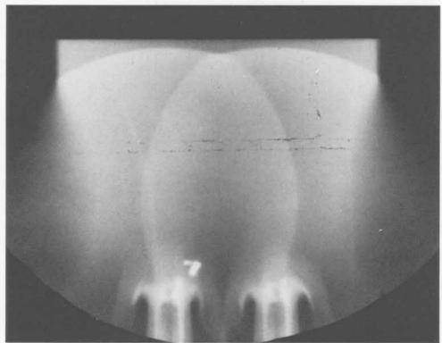
SHOT 1038: Colliding PBX-9404 Cylindrical Detonation Waves
