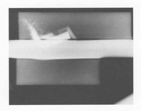
SHOT 1454: Projectile Penetration of a Steel Plate
