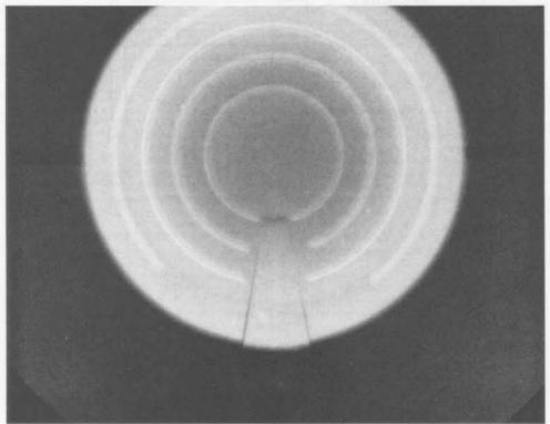
SHOT 989: Spherically Diverging PBX-9404 Detonation
