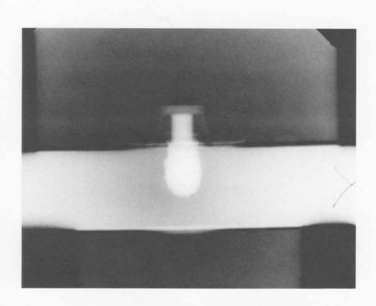
SHOT 1453: Projectile Penetration of a Steel Plate
