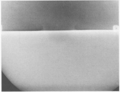
SHOT 1351: Water Splash Wave Formed by a PBX-9404 Sphere
