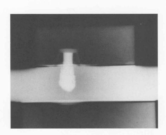
SHOT 1439: Projectile Penetration of a Steel Plate
