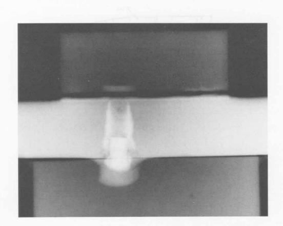
SHOT 1443: Projectile Penetration of a Steel Plate
