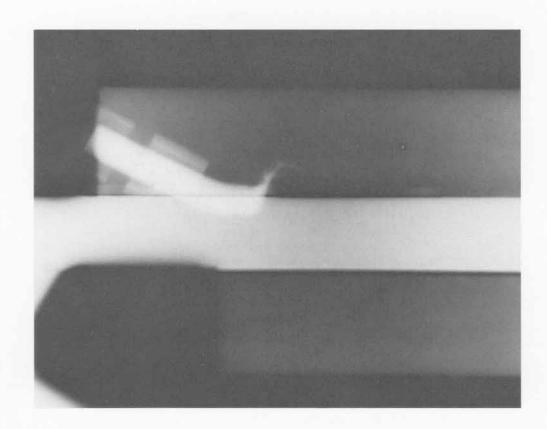
SHOT 1458: Projectile Penetration of a Steel Plate
