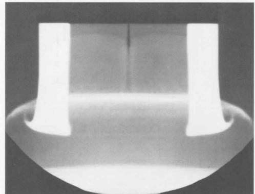
SHOT 1031: Spherically Diverging PBX-9404 Detonation
