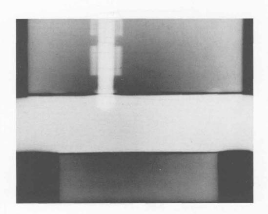
SHOT 1438: Projectile Penetration of a Steel Plate
