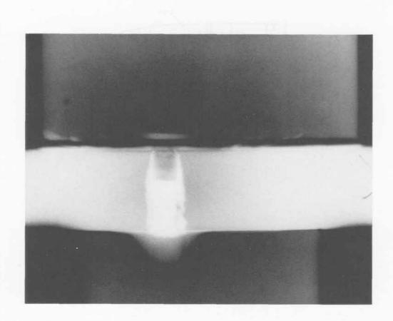
SHOT 1448: Projectile Penetration of a Steel Plate
