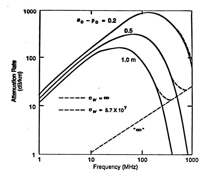
Attenuation rate of mode that behaves as axial surface wave at high frequencies for dielectric-coated conductor located in circular tunnel. Case indicated by " $\infty$ " corresponds to having conductor located in free space. For example shown, a=1mm, c=5mm,  $a_0=2$ m,  $a_0=2$ .56,  $a_0=1$ 0 = 4  $\times$  10<sup>7</sup>,  $a_0=1$ 0 = 1 mmho/m,  $a_0=1$ 0 = 5, and  $a_0=1$ 0 = 8.85  $a_0=1$ 0 is the distance of the conductor from the tunnel wall.
