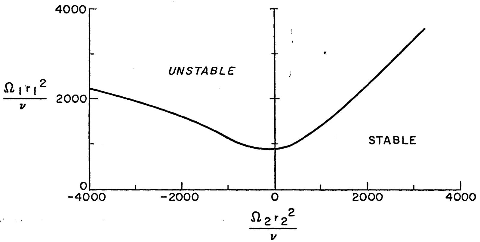
Fig. 1. Stability Diagram of Circular Couette.
