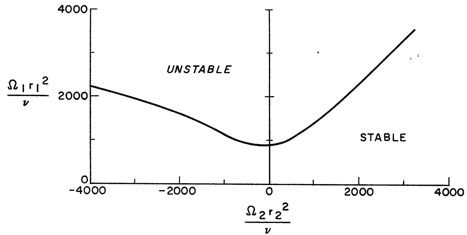
Fig. 1. Stability Diagram of Circular Couette.
