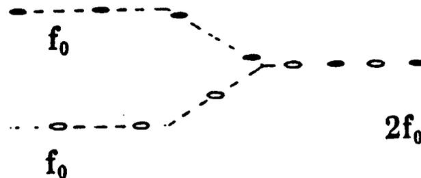
1. With funneling, two ion sources provide the required current at lower emittance.
