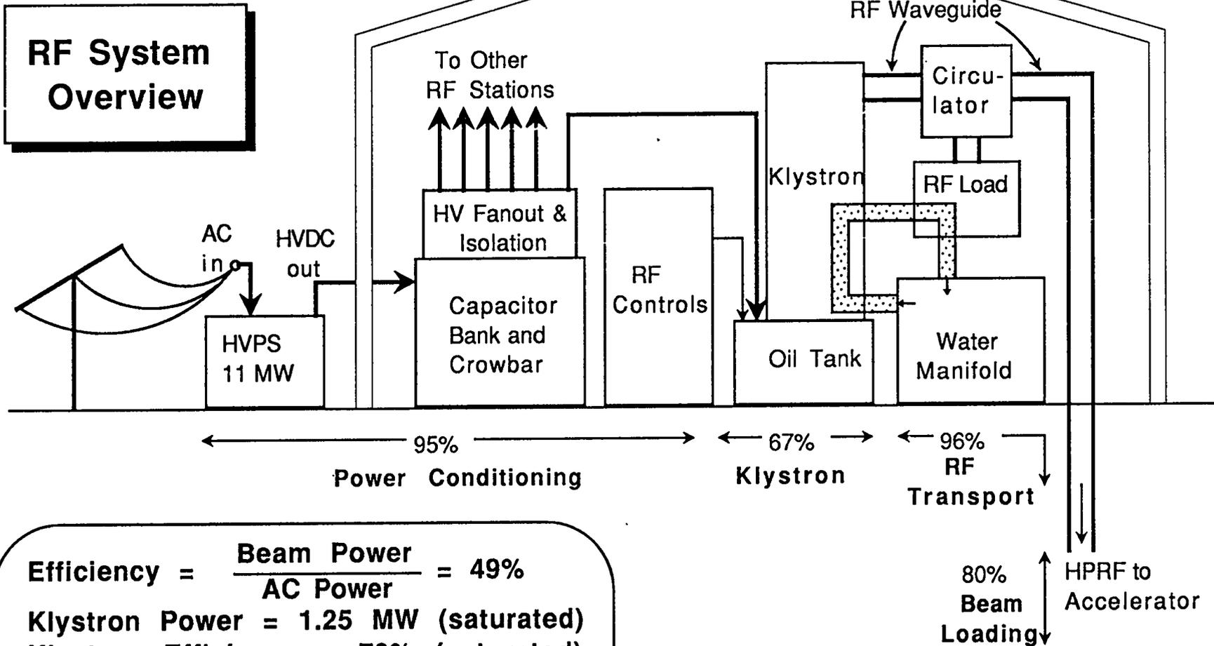
$$\text{Efficiency} = \frac{\text{Beam Power}}{\text{AC Power}} = 49\%$$
