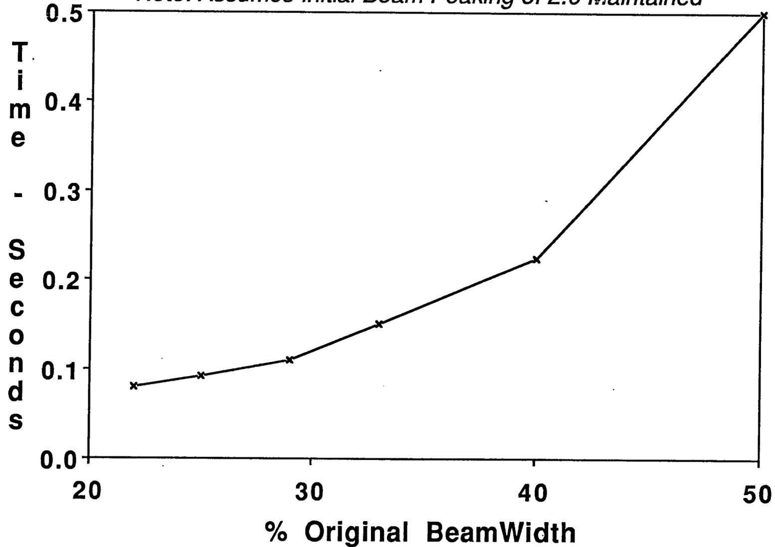
Conclusion: If Beam Can Be Inadvertently Focused in 20% Range, Must Assure Beam Trip In 50 milliseconds or Less (Feasible)
