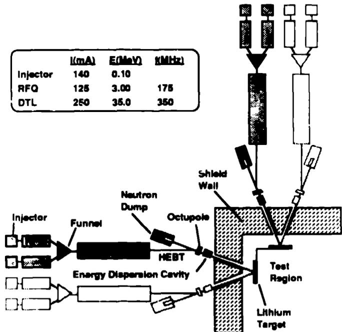
Fig. 1. Reference Neutron Source: Two 250-mA accelerator modules and two lithium targets. Lightly drawn modules indicate upgrade potential.
