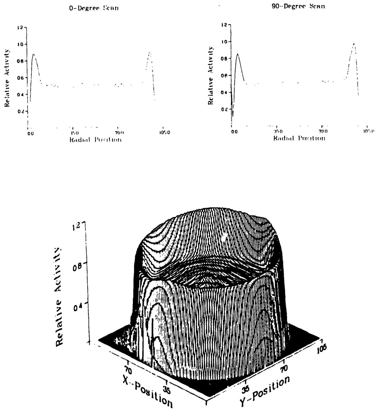
Figure 3: Reconstruction of the test case using the filtered backprojection technique.
