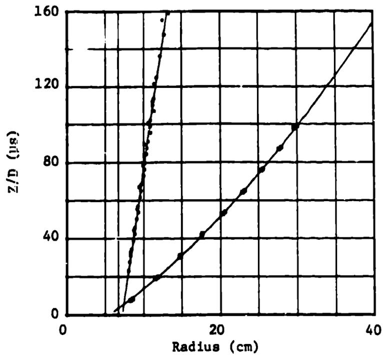
Fig. 2a. Shock front and pipe expansion data for aquarium test 4652 ( $\rho_0 = 0.90$  g/cm<sup>3</sup>) with least-square fits (solid lines).
