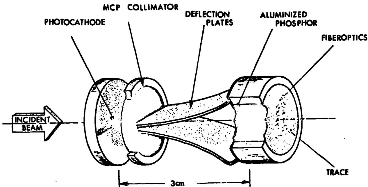
Fig. 1. Schematic proximity-focused streak tube.
