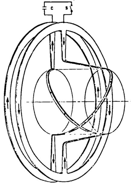
Fig. 1. Simple (two-conductor) Marshall coil showing current flow.
