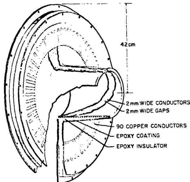
Fig. 4 Cutaway of the Prototype Marshall implosion coil.
