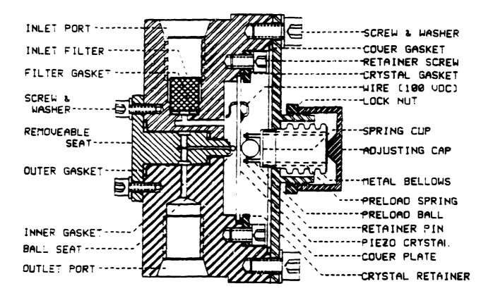
Fig. 1. The TFTR tritium-hardened piezoelectric valve.
