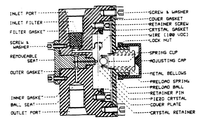
Fig. 2. Concept for a completely tritiumcompatible piezoelectric valve.
