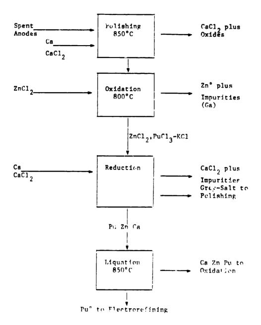
Fig. 2. Recovery of plutonium by pyroredox processing
