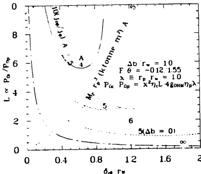
Fig. 2. Dependence of ohmic power losses in coils,  $P_{Oc}$ , relative to that in the plasma,  $P_{Op}$ , for a homogenized coil model, showing the dependence on plasma aspect ratio,  $A = R_p/r_p$ , poloidal coil thickness,  $\delta_{c0}$ , for a TFC standoff  $\Delta b = r_w$  and a minor radial plasma filling fraction  $x = 1$ . Shown also is the mass of the coil set,  $M_c$ , and the ratio of PFC to plasma current density,  $j_{c0}/j_0$ .
