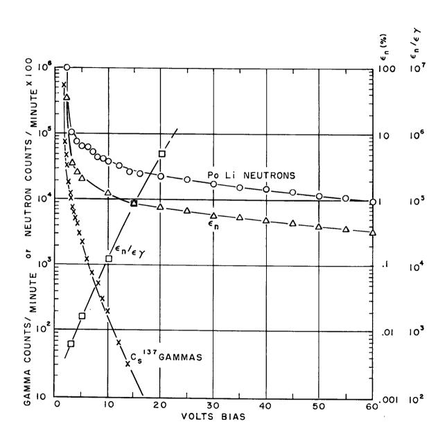
Fig. 8 Counting efficiencies as a function of bias voltage (background corrected).
