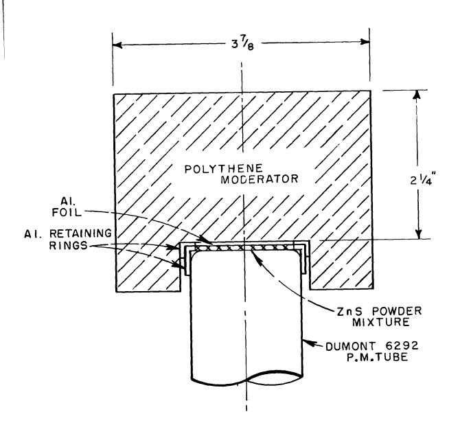
Fig. 4 Standard counting geometry and method of mounting phosphor mixtures.
