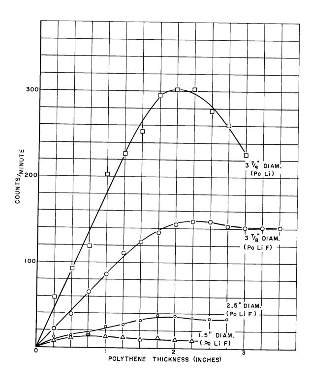
Fig. 3 Neutron counting rates for various polythene geometries.
