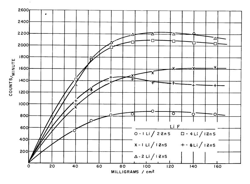
Fig. 5 Neutron counting rate vs thickness for various mixtures of ZnS and LiF.
