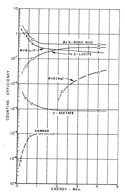
Fig. 7 Neutron and  $\gamma$  counting efficiencies as a function of energy for various optimum detectors in standard geometry.
