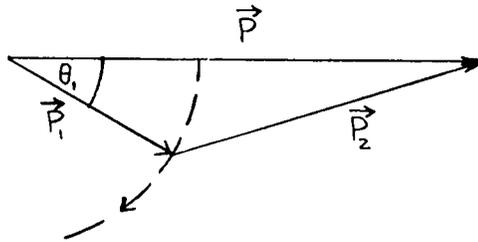
The idea behind the Williams' derivation, as applied to the variable  $E_1$ , is to find the total number of states with energy less than or equal to  $E$ , with fixed  $E_1$  and  $\vec{p}$  (and  $\varphi_1$ ), and then differentiate this expression with respect to  $E$  to find the number of states per unit total energy.
