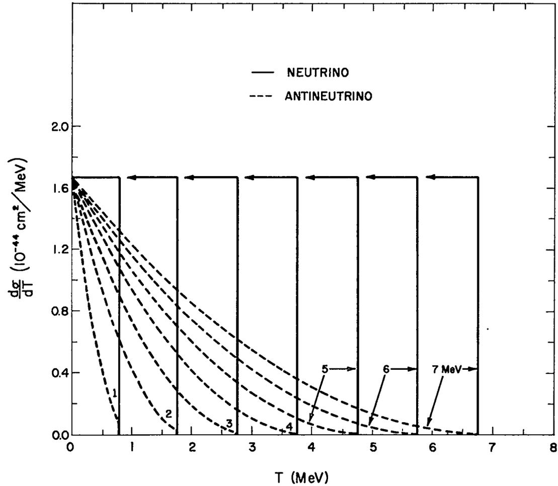
Figure I. Laboratory differential cross section per unit electron recoil kinetic energy  $T$ , vs  $T$ , for elastic neutrino and antineutrino scattering on electrons. The curves are labeled by the incident neutrino or antineutrino laboratory energy in MeV. Note that the electron recoil spectrum is flat from  $T = 0$  to  $T_{\text{max}}$  for the case of incident neutrinos. The calculation assumes that there are no neutral symmetric currents.
