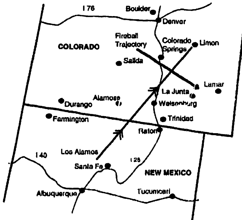
Figure 4. A map of the region in which the fireball entered the Earth's atmosphere and the corresponding infrasonic azimuth computed assuming a plane wave across the Los Alamos, New Mexico array.
