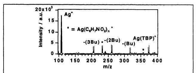
Figure 2: The Ag(2+1) RLA mass spectrum for a silver modified zeolite equilibrated with TBP headspace vapors. The zeolite was mounted on a type 304L Stainless steel probe with Ethyl-Cyanoacrylate Glue.
