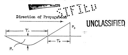
The figure indicates the characteristic shape possessed by the blast front. This the duration of the positive (The of the negative) phase.
