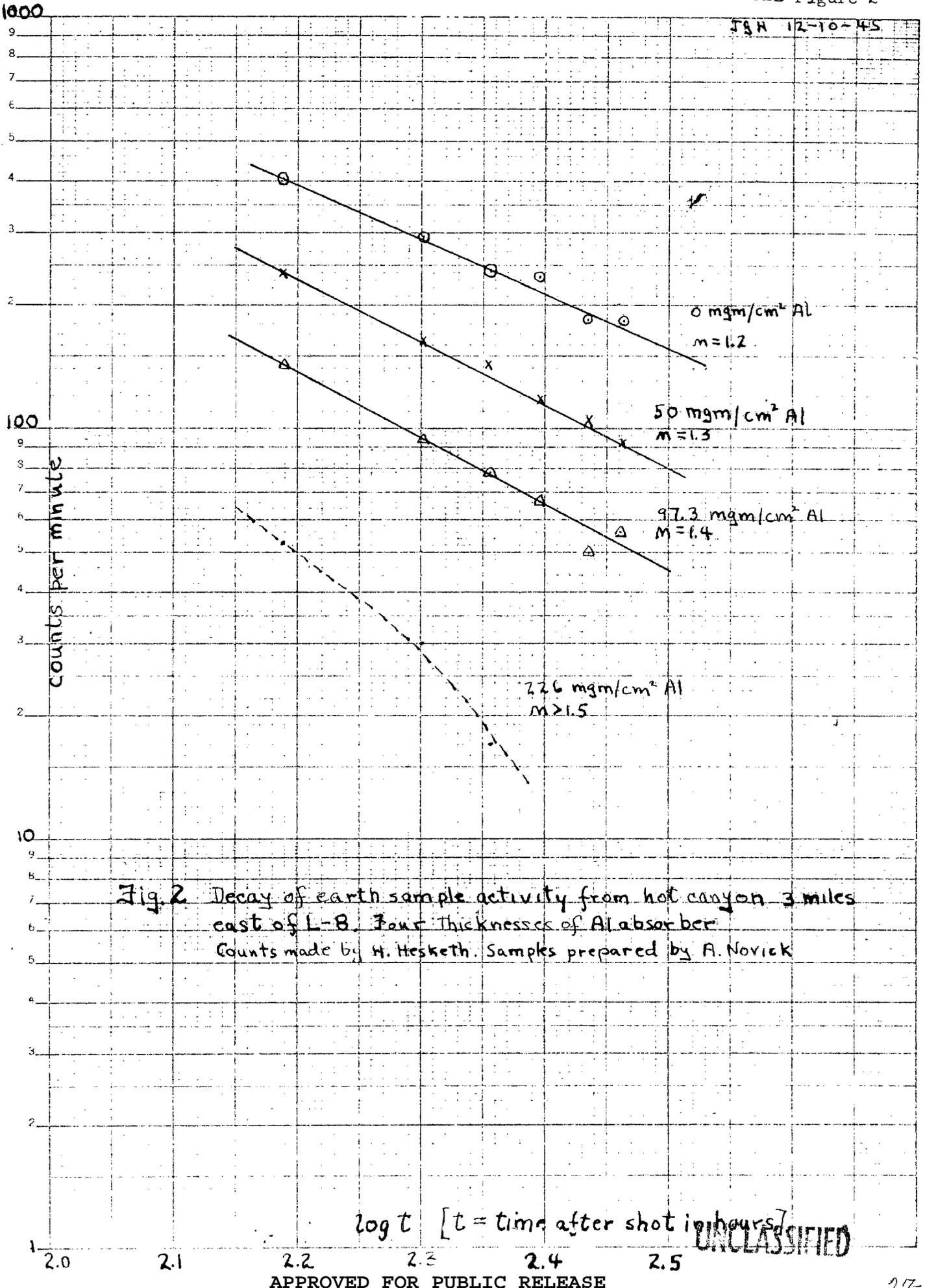
Fig. 2 Decay of earth sample activity from hot canyon 3 miles east of L-8. Four thicknesses of Al absorber. Counts made by H. Hesketh. Samples prepared by A. Novick
