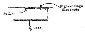
Therefore the chamber used in these measurements was made quite deep; the distance between the plates, c, on either side of the high-voltage electrode was 1.5 cm.
