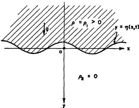
Fig. 5. Physical arrangement for problem described by Eqs. (3.1).
