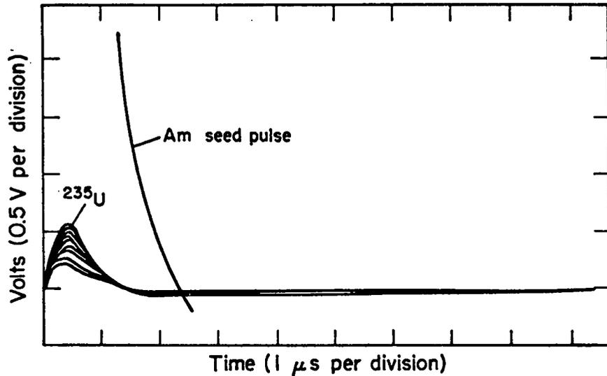
Fig. 3.4. Oscilloscope display of <sup>235</sup>U gamma-ray pulse from a SAM II.
