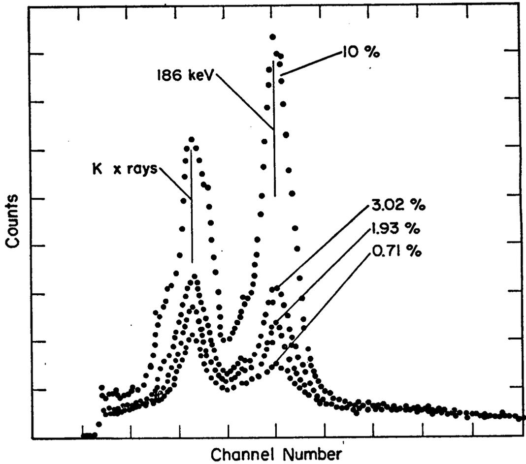
Fig. 3.3. Pulse-height distributions of four different enrichments of uranium oxide.
