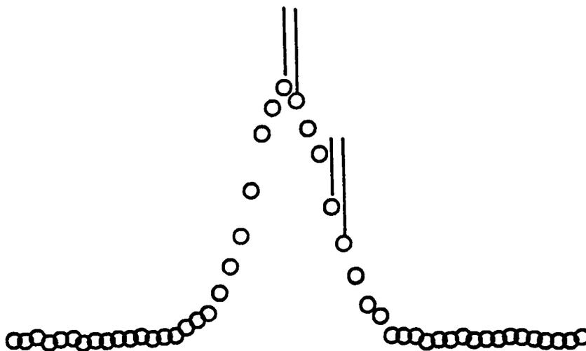
Fig. 1.3. Count rate changes near peak and 1/2-max point. The same gain shift (indicated by the vertical bars) produces a much larger change in count rate near the 1/2-max point.
