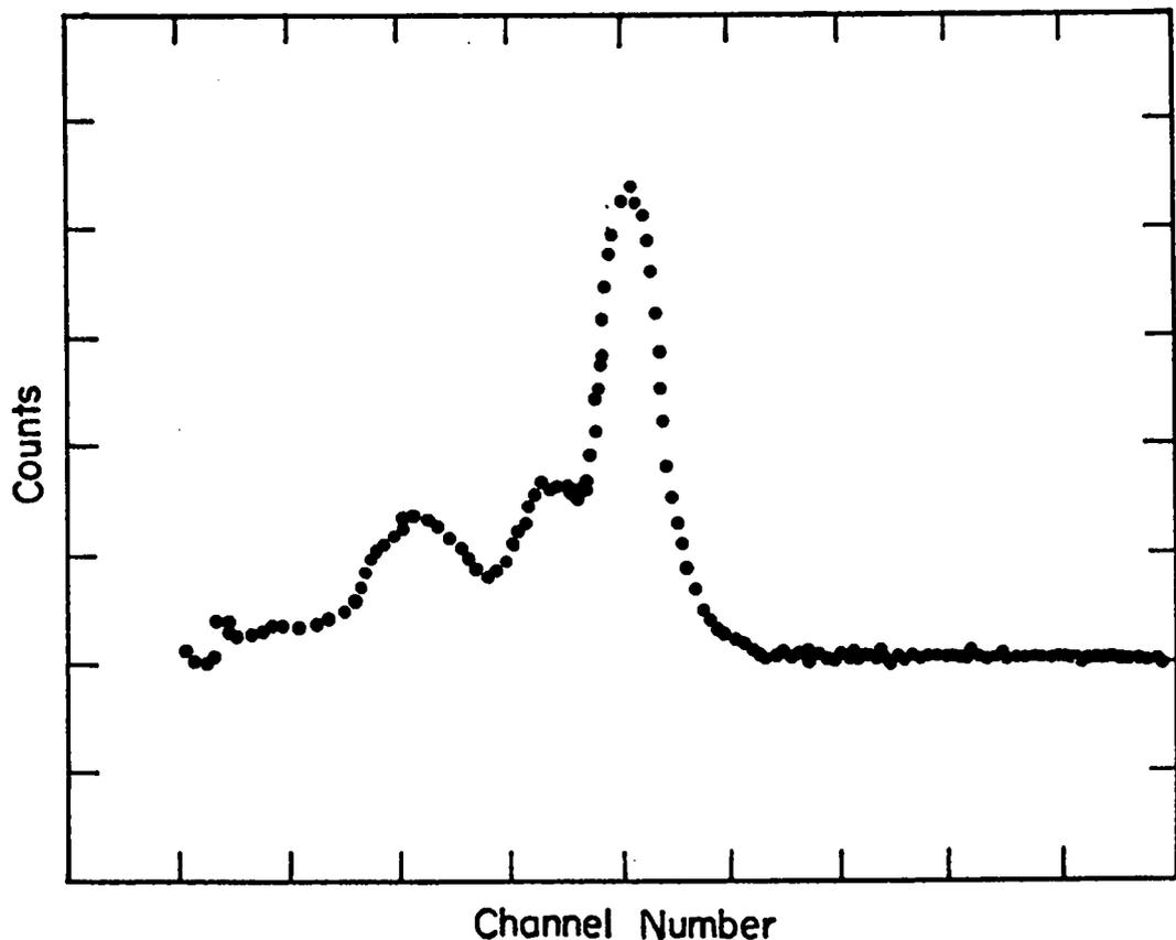
Fig. 3.2. Pulse-height distribution of 93% enriched uranium metal foil.
