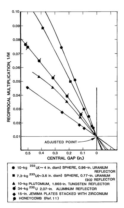
Fig. 1. Typical relations between reciprocal multiplication and gap on median plane; adjusted to M = 100 at zero gap.
