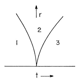
Fig. 1-1 r-t trajectories of incoming and reflected shocks.
