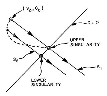
Fig. 6-1 The dashed line is the locus of points accessible from  $\rm S_1$  by the jump conditions.
