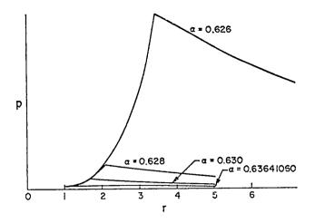
Fig. 3-3 Pressure profiles for  $\gamma = 3$ , spherical symmetry.
