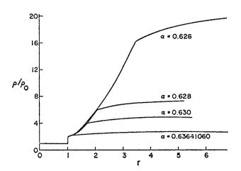
Fig. 3-4 Compression profiles for  $\gamma = 3$ , spherical symmetry.
