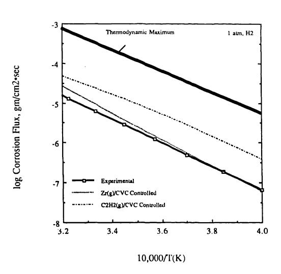
Figure 1. Arrhenius plot of corrosion flux comparing measured and calculated rates.
