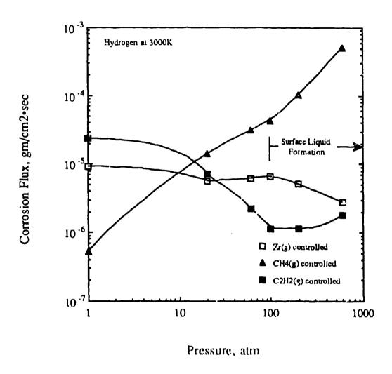
Figure 2. Calculated corrosion flux versus hydrogen pressure under three assumptions: that corrosion is rate limited by the gaseous transport of Zr,  $CH_4$ , and  $C_2H_2$ .
