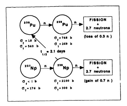
Fig. 3. Diagram illustrating two-step process for thermal burning of threshold fissioning actinides. The upper branch dominates at low fluxes.
