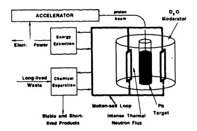
Fig. 2. Schematic diagram illustrating the Los Alamos concept for energy production and waste transmutation. The proton beam generates neutrons from a lead target which are moderated in the heavy water blanket. Molten salt circulating through the blanket carries fissile material for heat generation and power production. Nuclear waste is also circulated through the blanket and transmuted to stable and short-lived nuclides which are then chemically extracted.
