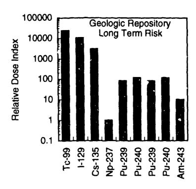
Fig. 1. Relative Radiation Dose Index for Some Fission Products and Actinides during geologic storage. From Ref. [6].
