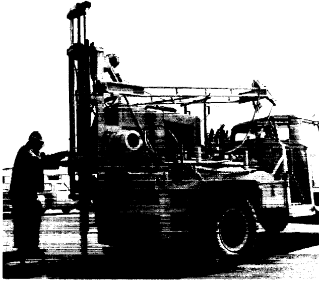
Fig. 17. Truck-mounted, auger-drill rig.
