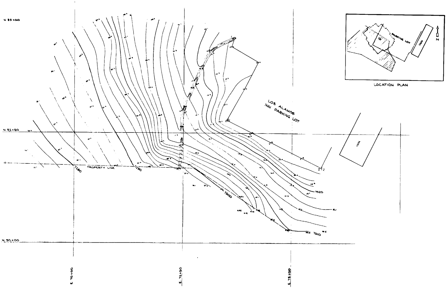
Fig. 62. Contour map of final grading in the D and D-2 areas.
