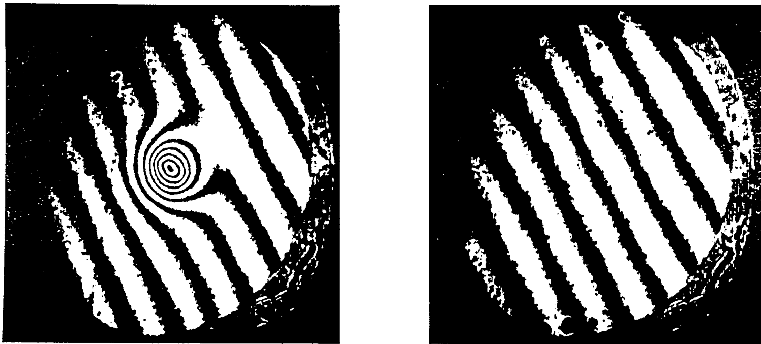
Fig. 4. Compressed plasma of the Los Alamos Scylla IV \theta pinch as shown by Mach-Zehnder interferogram at \lambda = 6943 \text{ \AA} . This is near peak compression in the new low pressure, higher temperature regime without reverse magnetic field heating. P (initial) = 15 m-torr D_2 . B applied = 90 kGauss. Time = 1.6 \mu\text{sec} . Plasma mean length = 70 cm. 1 fringe = 3.10^{17} electron/cm 2 . Mean ion energy (calc) = 7.3 keV (equivalent to 4.9 keV ion temperature for Maxwellized ion energies). Electron temperature = 300 eV. Mean neutron yield = 6 \times 10^8 per discharge. Note absence of wall impurities.
