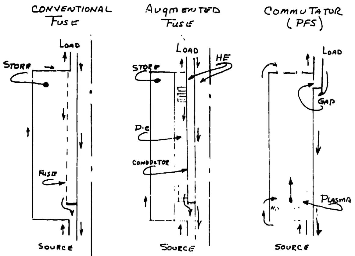
FIGURE 2 Configurations for High Current Opening Switches
