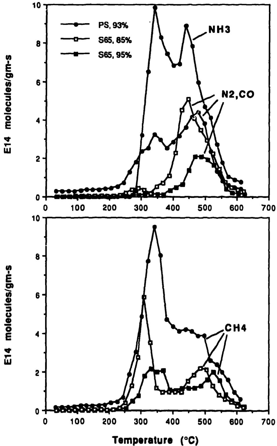
Fig. 9. Comparison of the  $\text{N}_2/\text{CO}$ ,  $\text{NH}_3$ , and  $\text{CH}_4$  desorption spectra for plasma sprayed (PS) and S 65 materials of the indicated densities.
