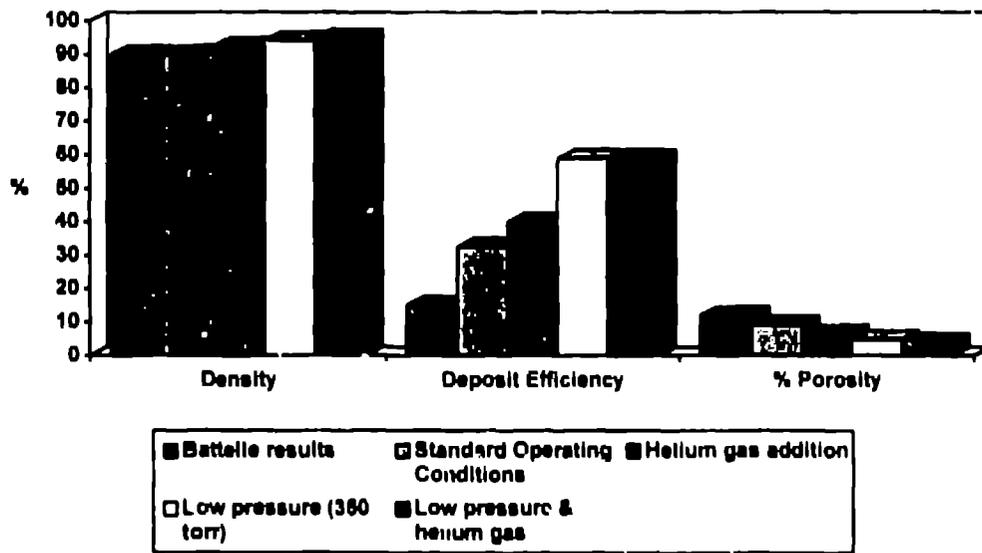
**Fig. 4.** As deposited density, deposit efficiency and porosity level of plasma sprayed ( $30\mu\text{m}$ ) beryllium powder sprayed under the various operating conditions and compared to results previously reported by Battelle, Columbus [8].
