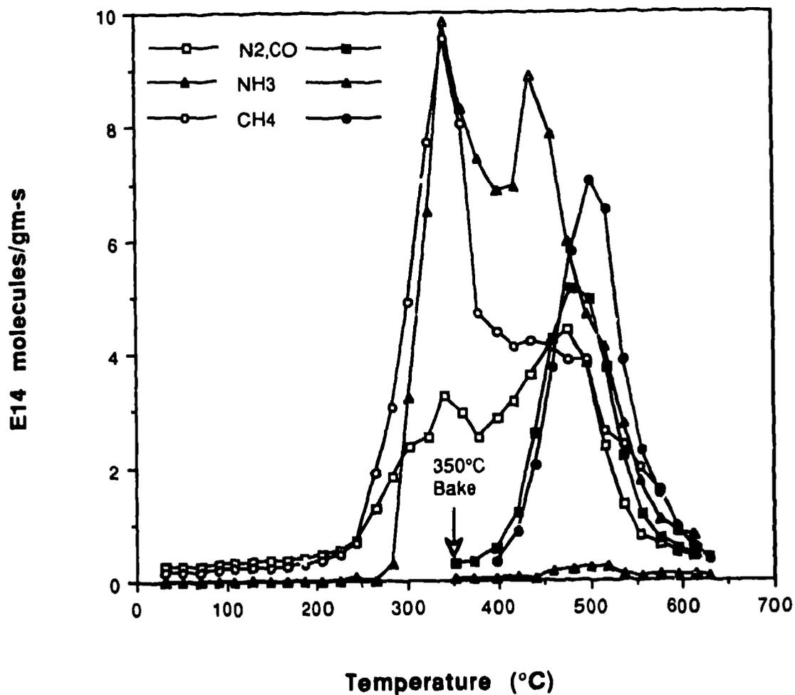
Fig. 10. Comparison of desorption spectra for (P5) material pre baked at 350°C for 90 minutes with unbaked material. Pre baking removed the water peak but not the water outgassing.
