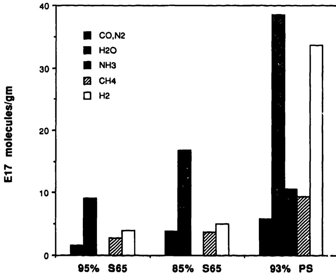
Fig. 7. Quantities of gases produced by heating as received plasma sprayed (PS) and S 65 materials of the indicated densities.
