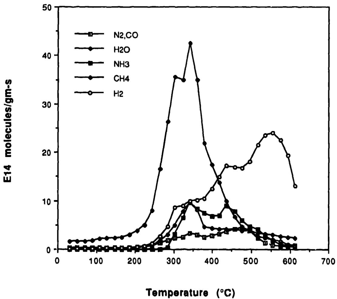
Fig. 8. Gas desorption spectra from 94% dense plasma sprayed beryllium samples.
