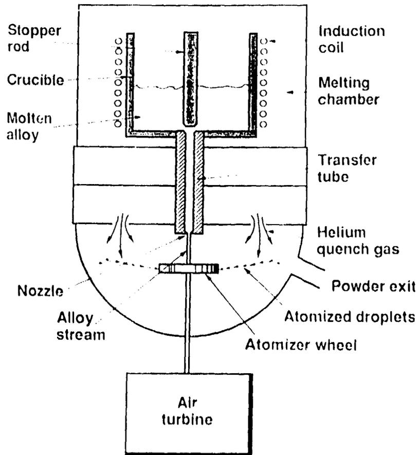
Fig. 1. Schematic of centrifugal atomization process.
