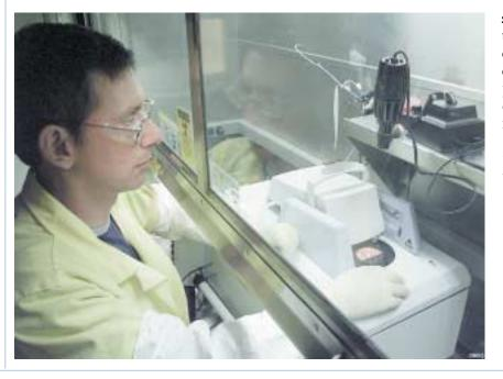
In power-compensated DSC, this causes the instrument to increase power input to compensate, until the phase transition is complete. The DSC instrument in the CMR Building is capable of measuring with high purity standards the onset temperature for phase transitions to an accuracy of plus or minus 0.05 degrees Celsius, and heat capacity and enthalpy to plus or minus 2 percent.
