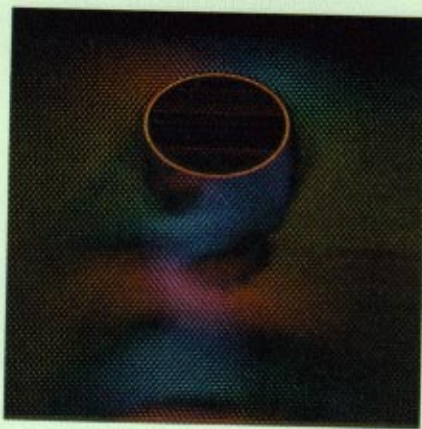
Fig. 5. A turbulent wake grows behind an ellipse being dragged through a fluid consisting of 11 million particles and 8 million cells. The ellipse is composed of about 2400 cells in which the velocity directions of the entering particles are reversed. The flow has periodic right and left boundaries. (An infinite sequence of equivalent ellipses exists to the left and right of the frame shown.) The Reynolds number in the flow is 1021.
