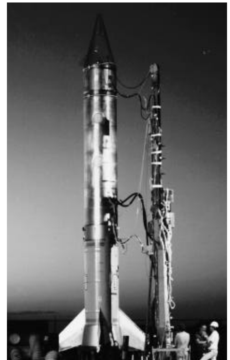
Aries Rocket at White Sands Missile Range. This type of rocket carried into space an accelerator for producing a neutral-particle beam.
