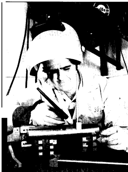
Chris Espinoza welding heat exchange manifolds onto the resonator tube of the liquid sodium natural heat engine.
