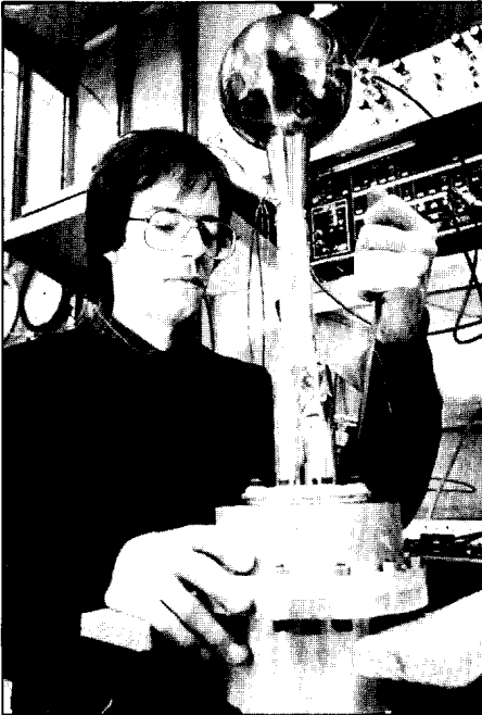
Tom Hofer attaching the resonator of the cryocooler to the housing of the cooler's driver and hot heat exchanger.
