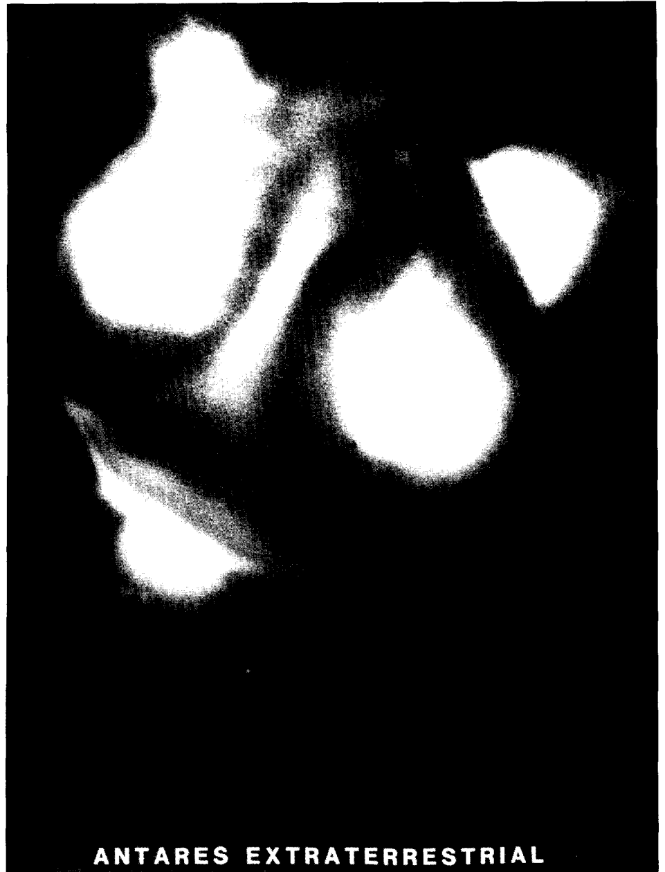
Fig. 18. An \sim 1 -keV x-ray image of the surface of a target being hit simultaneously by the six laser beams of Antares. The narrow region of x-ray emission at the center of the photo is evidence of strong magnetic fields encircling each laser spot; here the fields from adjacent spots cancel, allowing the electrons to move freely into the target rather than being trapped above the surface.
