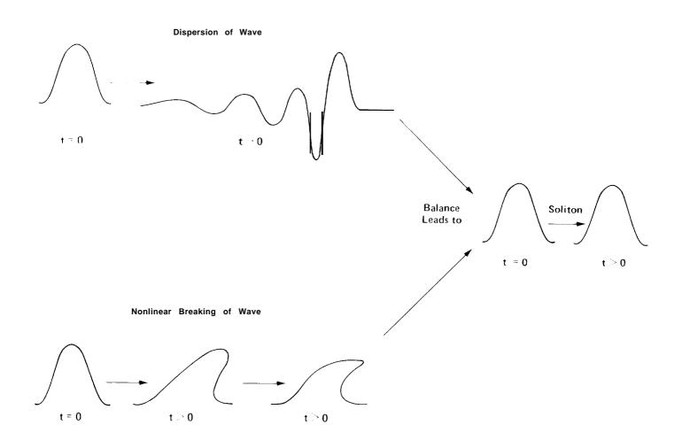
Fig. 1. Two effects, dispersion and breaking, cause the shape of a wave to change as it propagates. For a wave described by
