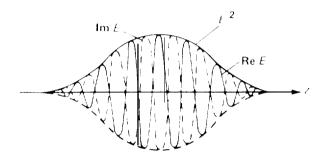
Fig. 2. Profile of a single-soliton solution of the NLS equation.
