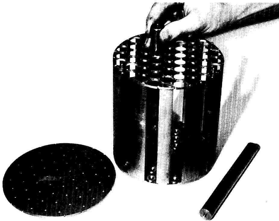
Fig. 5. Clementine fuel rod cage, constructed of mild steel. Mercury coolant circulated through the cage.
