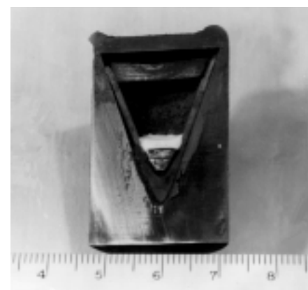
The plutonium compound was placed inside a graphite crucible and was then reduced in the centrifuge. The longitudinal cross-section view above shows the button of plutonium metal obtained after reduction.
