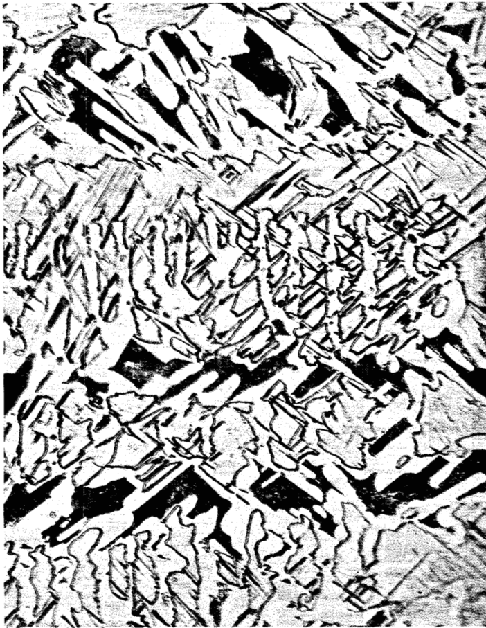
With further increase of yttrium [at left, this page ( Y_{.25}Ir_{.75} )] the amount of eutectic begins to decrease; the light areas are probably YIr_2 . At the right ( Y_{.30}Ir_{.70} ), the eutectic, the dark bubble-like structures, has almost disappeared. The lighter areas are YIr_2 . The amount of eutectic for each composition is proportional to the percentage of material that is superconducting as measured by specific heat measurements. (1000X) Metallography by Ramiro A. Pereysa.
