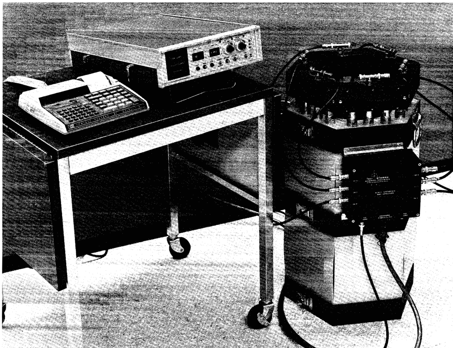
Fig. 4. The high-level neutron coincidence counter (HLNCC) detects neutrons from the spontaneous fission of ^{240}\text{Pu} using ^3\text{He} proportional counters in a polyethylene moderator. A shift register coincidence technique is used to distinguish fission neutrons from background. The instrument is portable for use by IAEA inspectors. The electronics to operate the detectors and analyze the coincidence data are contained in the package on the table, next to a programmable calculator that is interfaced to the shift register unit.
