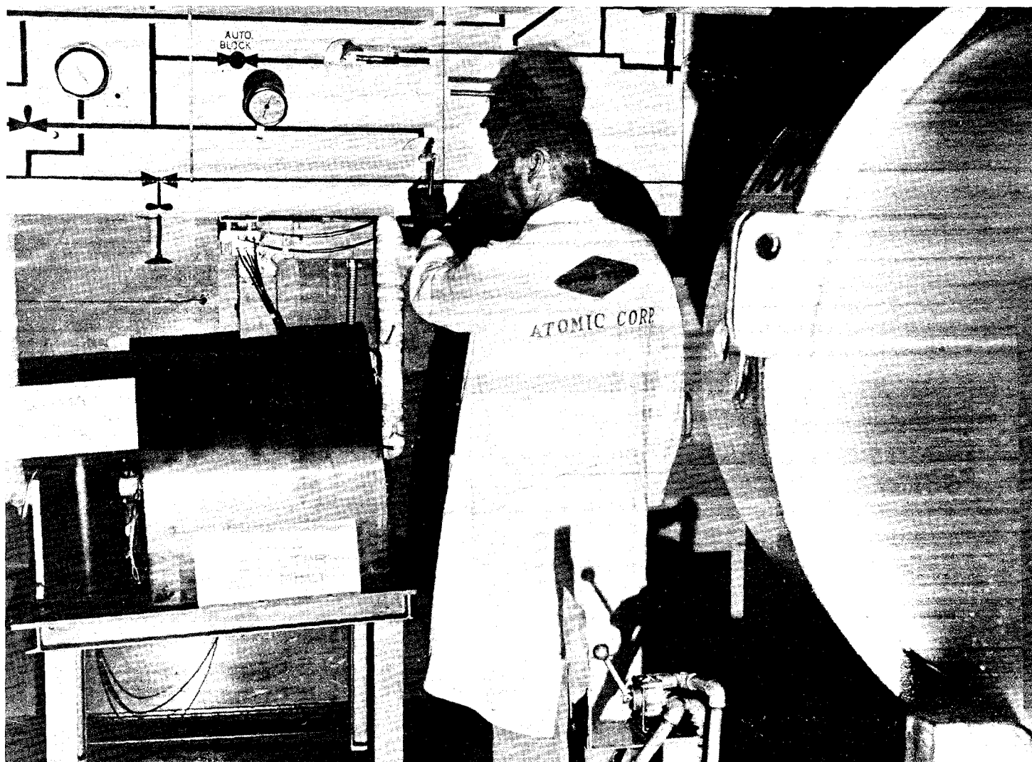
Fig. 21. In-line UF_6 enrichment monitor installation at the extended-range product-withdrawal station of the DOE/Goodyear Atomic gaseous diffusion plants. Passive gamma-ray and neutron instruments continuously measure ^{235}U and ^{234}U enrichments of liquid UF_6 to provide criticality safety and process controls.
