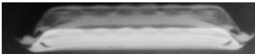
Figure 6. Double-Pulse PHERMEX Radiograph of Spall in Iron
